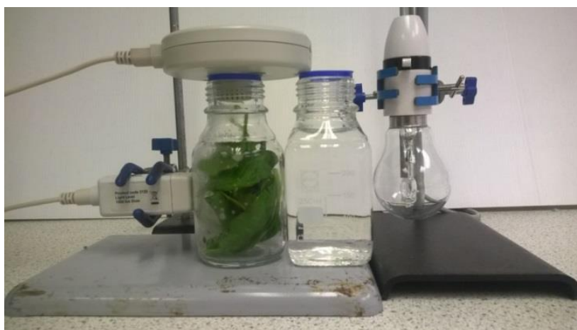
Fig 15d.1 Photograph of typical bench layout of apparatus, the light source would be removed for respiration studies as could the heat sink. We did find that turning the light on was a convenient way of bringing the CO 2 levels round the leaves back down to a lower value again.
