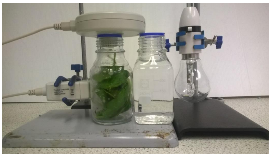
Fig 15a.1 Photograph of typical bench layout of apparatus, the light source would normally be bench lamp. Note the position of the optional Light sensor.
