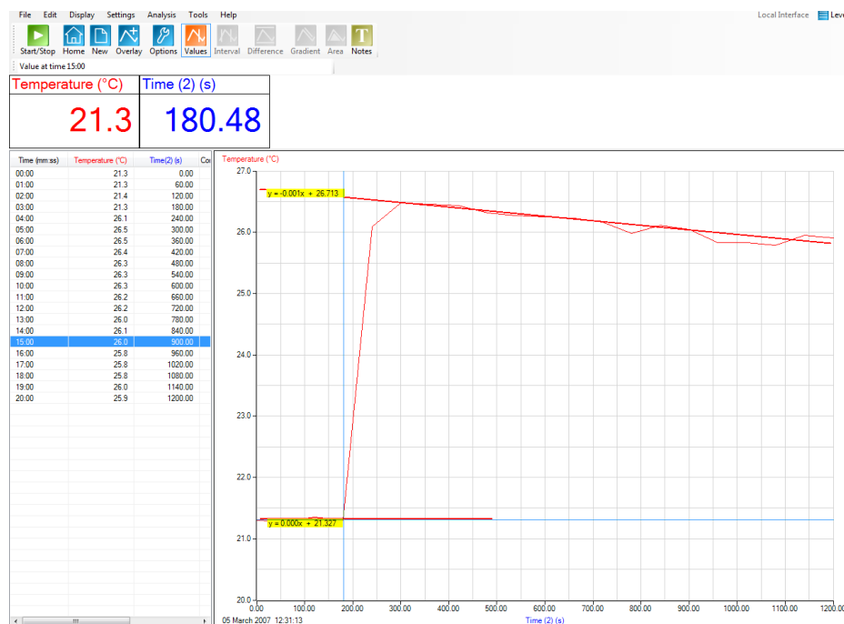
Fig 3.8 Using the Values tool to find the T_2 value, align with the same Time(2) used for the T_0 value and set the horizontal values line onto the upper best fit line.
