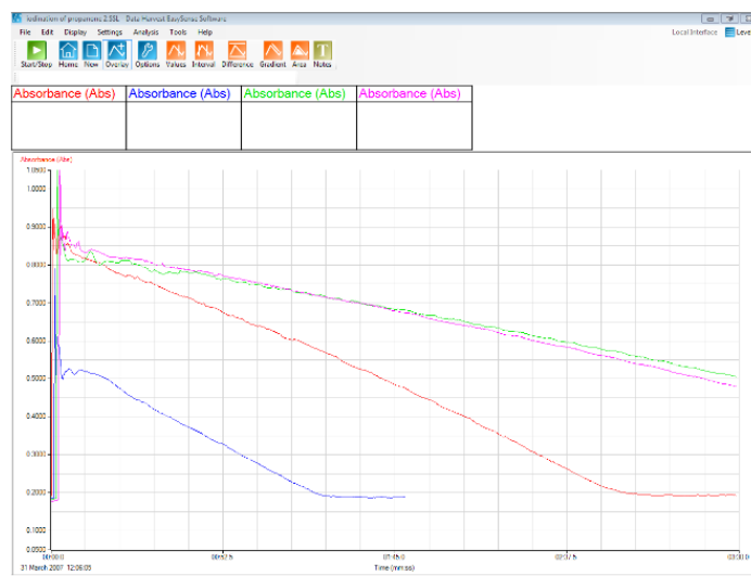
Fig 12.1 Example of a complete set of data. Note the erratic data at the beginning of each of the recordings, this is the change in light due to the addition of the iodine, this has no significance as we are interested in the rate.
