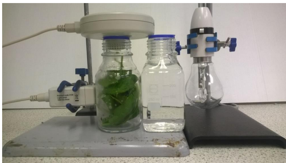
Fig 15c.1 Photograph of typical bench layout of apparatus, the light source would normally be bench lamp. Note the position of the Light level sensor
